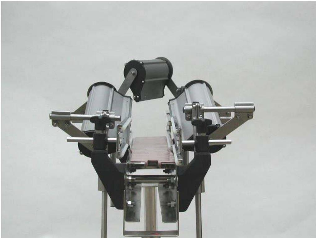
**Figure 12 - Air Knife Installation - Front View**
