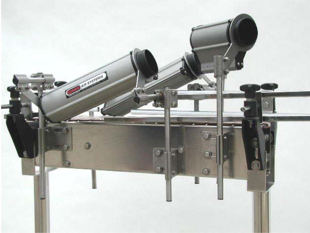
**Figure 11 - Air Knife Installation - Side View**
