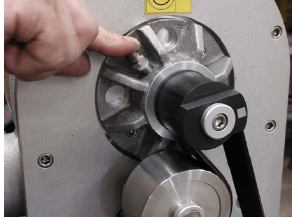
2) Apply Teflon Tape and install Sensor Pipe Fitting
